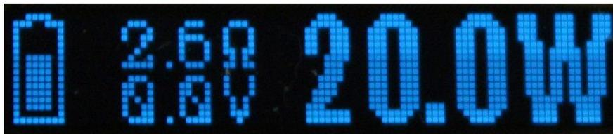
The DNA 20D has a small .69" diagonal blue OLED screen. The screen is attached to the main board by a flexible cable, allowing freedom in the design of your device. Please use caution when handling the screen and design the device so that the cable will be secured or strain relieved in operation. The normal and special operating modes shown on the display are discussed below.
